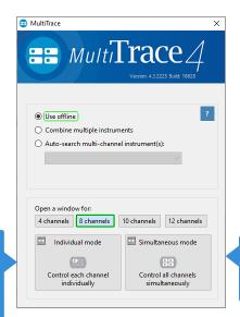
Individual Mode: where each channel can run a measurement or script independently from the other channels.
